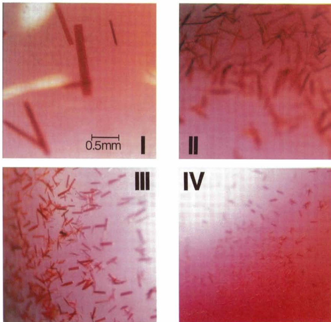
Fig. 3. Photographs showing the effect of PEG concentration on the crystal size of PRCs from R. sphaeroides . C_0 was 3.3 \text{ mg ml}^{-1} , PEG concentrations were: 15.0 (I), 16.3 (II), 17.5 (III) and 18.8% (w/v) (IV) as shown in Fig. 1.
